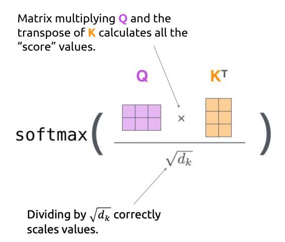
The result is a **Z** matrix where Matrix multiplying Q and the the i<sup>th</sup> row represents the transpose of K calculates all the self-attention vector  $\mathbf{z}$ , "score" values. × Multiplying the resulting Dividing by  $\sqrt{d_k}$  correctly vector with **V** properly scales values. weighs the v, vectors.
