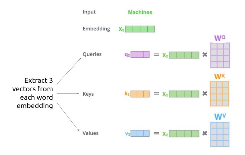
Each vector is obtained by multiplying the embedding with the respective weight matrix.
