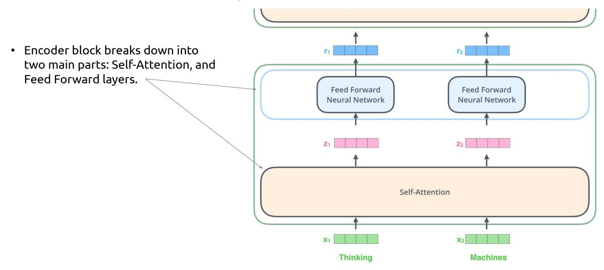
Encoder block breaks down into two main parts: Self-Attention, and Feed Forward layers.
